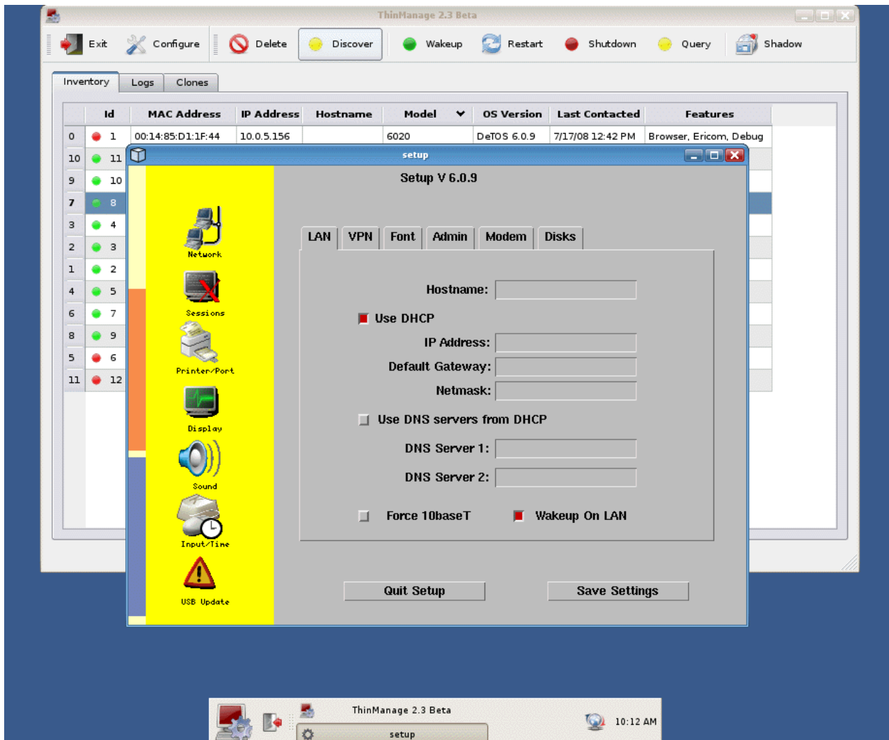
Figure 3-5: Screenshot of a DeTOS Setup window that displays after a “Remote Configure” is initiated.
