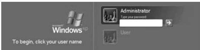
Figure A – Hold the Shift key during bootup or logoff to access the Windows XP Logon Screen
